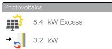
Current PV surplus and current power consumption of the heat pump
