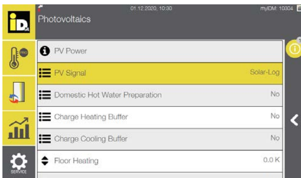
PV signal „Solar-Log“ navigator control setting
